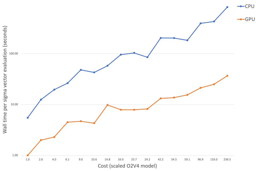
Figure 4: Scaling of sigma vector evaluation for benchmark calculations employing CPU and GPU offloading for increased problem size (on the basis of the scaled cost measure, see table 9).
